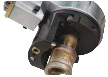
Axial slide for socket weld removal
