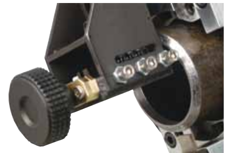
Counterbore attachment fits all models. Mounts securely to tool slide.
