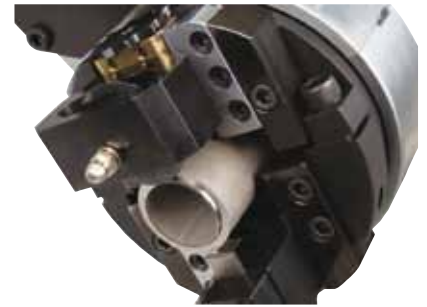
Wheel cutting module for FME cutting
