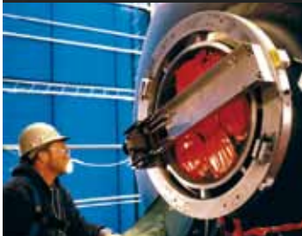
Optional "Bridge Slide" for heavy wall pipe. Bevel, compound bevel and J prep.
