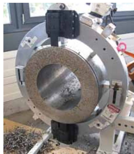
LCSF with worm slide assembly
