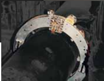
All "Low Clearance Split Frames" are designed for portability and are applicable even where space is limited.
